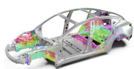
Model 3 body structure 171 pieces of metal highlighted
