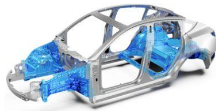
Austin-made Model Y body structure 2 pieces of metal highlighted >1,600 fewer welds
